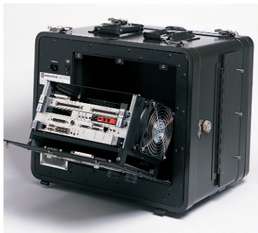
6-slot swing-out VME card cage
